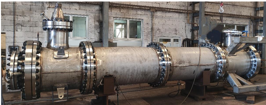
Figure 9: Reactor under construction
