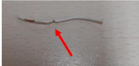
Figure 25: Replaced cable for the water-air cooling system
