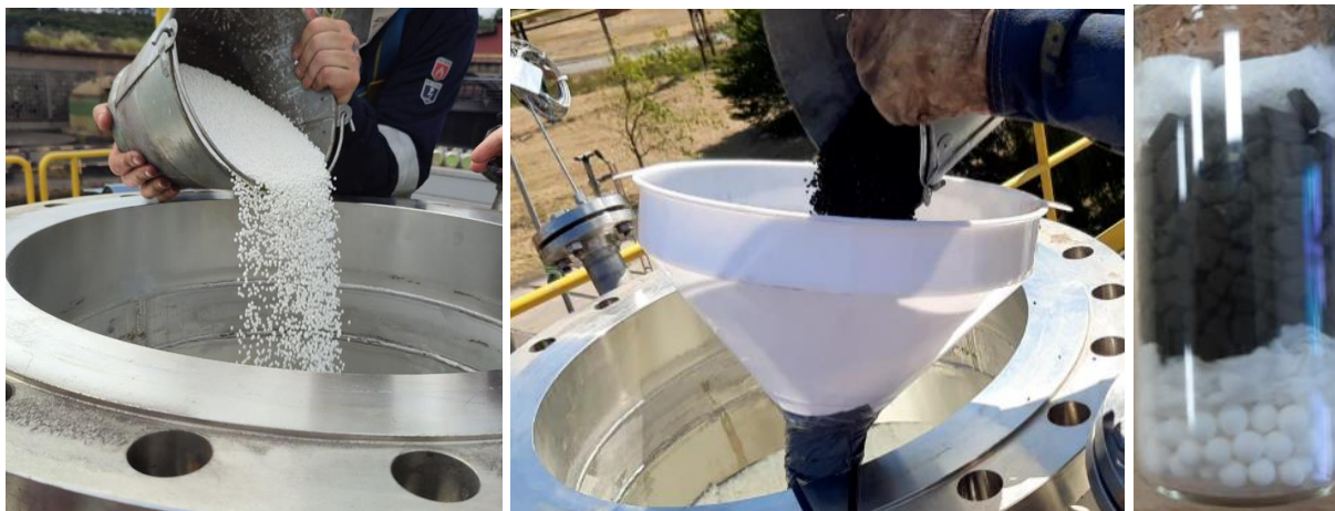
Figure 20: Material loading in the reactor (left and middle) and reactor material structure (right)
