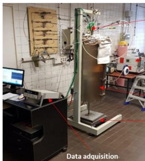
Figure 8: Experimental set up at CSIC-INCAR used to conduct the initial vacuum calcination tests using large limestone particles ( d_p=20 mm)
