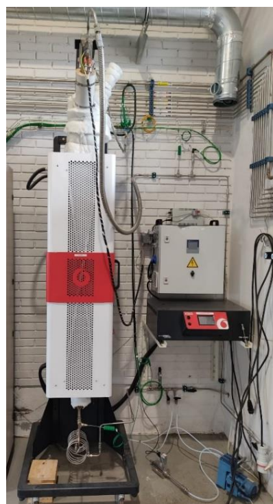
Figure 12. Left: Experimental set up at CSIC-INCAR used to conduct vacuum calcination test of the limestone chosen for TRL7 testing. Right: experimental temperature profiles.
