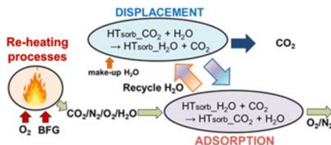
Figure 2: Schematic representation of the DISPLACE process.
