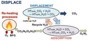
**DISPLACE** – high-temperature sorption-displacement process for CO<sub>2</sub> recovery
